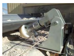
Option « BT » for mounting underneath the conveyor
