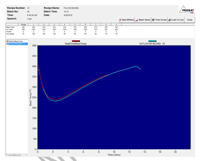
This screen allows the operator to view the curve, roast data, and recipe data from previously roasted batches. A report for a specific batch is available for selection once that corresponding batch has been released from the Destoner hopper.
