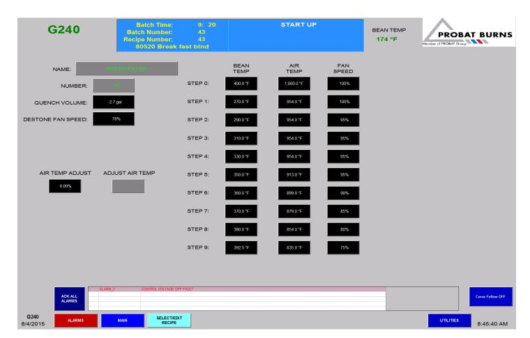
This display is the *RECIPE* screen, with the proper Login, and Enable Edit Recipe engaged. This allows the user to modify values in a recipe and will be saved directly to the database.
