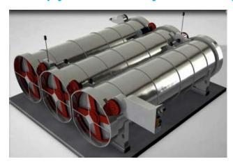
The JBT Rotary Pressure Sterilizer is a continuous machine where, at one side, the unsterilized cans enter the machine and at the other side the sterilized and cooled cans leave the machine in a continuous way.
